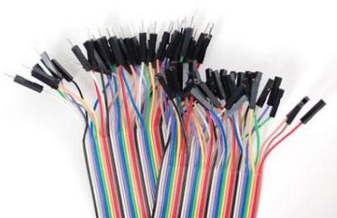
AVR micro. Male to male prototyping wires are very handy for making these point-to-point connections.
